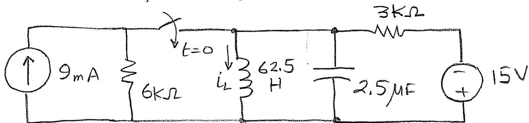
The switch has been in the open position for a long time. It is closed at  $t=0$ . Find  $i_L(t)$  for  $t \geq 0$ .
