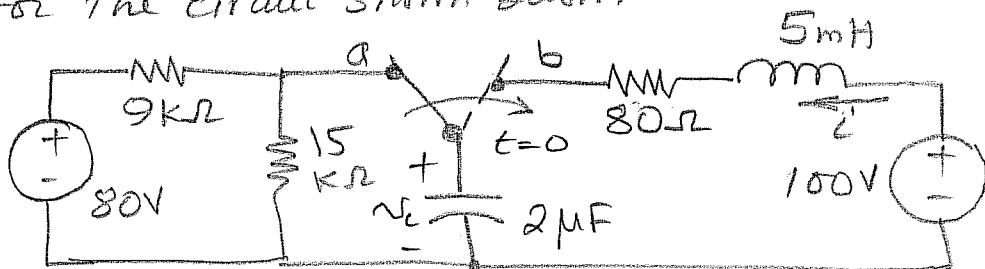
The switch has been in position a for a long time; at  $t=0$  the switch moves to position b.
