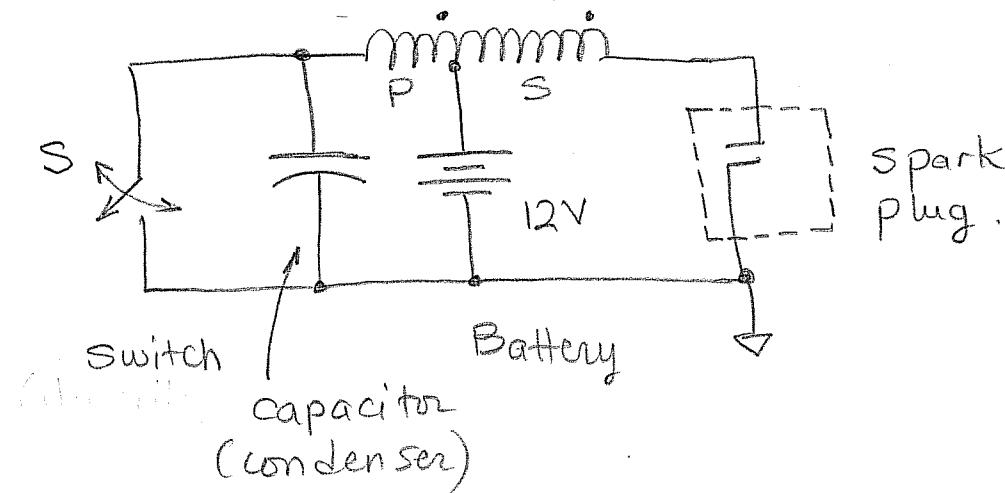
The switch S causes a rapidly changing current in the primary winding (P) which induces a very high voltage in the secondary winding (S) up to 40 kV, which will ignite a spark across the gap of the spark plug. In older cars the switch was a relay, whereas in today's cars the switch is electronic rather than a mechanical relay.
