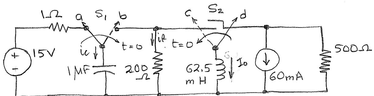
Switches  $S_1$  and  $S_2$  have been in positions a and d for a long time. At  $t=0$  both switches move to positions b and c, respectively. Find  $v(t)$  for  $t \geq 0$ .
